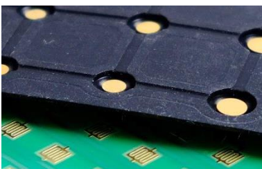
Gold pill with gold plated PCB contact
